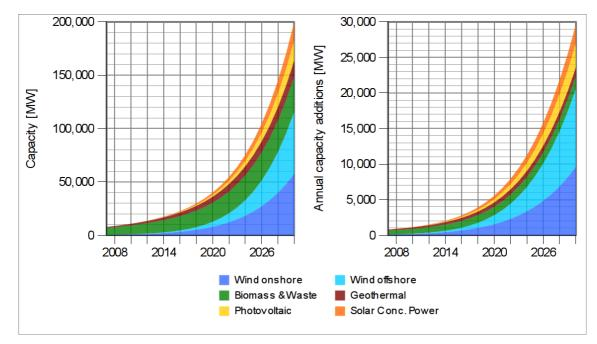
*Figure 53: Development of renewable electricity generating capacity in Latin America ("High Variant") [EWG; 2007].*
