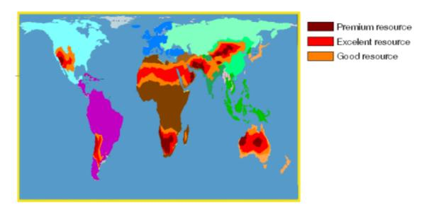
Figure 92: Solar thermal Power resources mapped to the "Peters projection" (showing true surface area), disaggregated into the regions used by the IEA [EWG; 2007].
