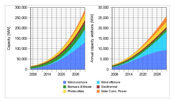
*Figure 38: Development of renewable electricity generating capacity in OECD Pacific ("High Variant") [EWG; 2007].*
