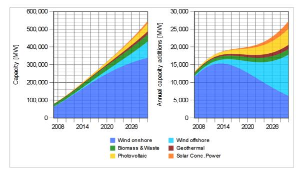
*Figure 62: Development of renewable electricity generating capacity in OECD Europe ("Low Variant") [EWG; 2008].*
