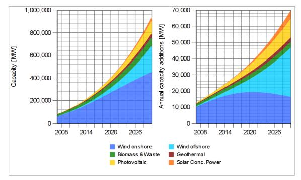
*Figure 32: Development of renewable electricity generating capacity in OECD Europe ("High Variant") [EWG; 2007].*
